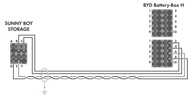
Figure 11: Cabling plan SBS3.8-US-10 / SBS5.0-US-10 / SBS6.0-US-10 with BYD Battery-Box H  $\,$
