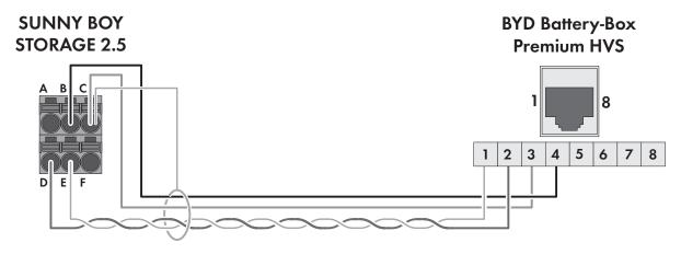
Figure 3: Cabling plan SBS2.5-1VL-10 with Battery-Box Premium HVS
