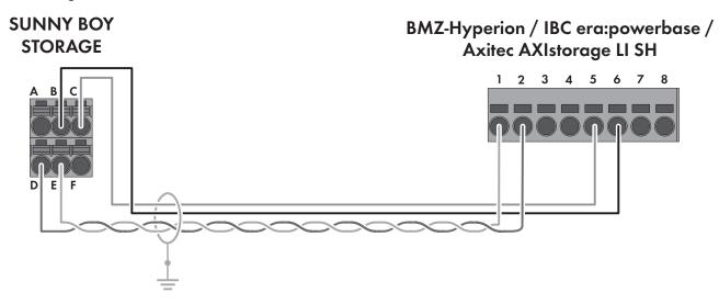
Figure 9: Cabling plan SBS3.7-10 / SBS5.0-10 / SBS6.0-10 with BMZ Hyperion, IBC era:powerbase and Axitec AXIstorage Li SH
