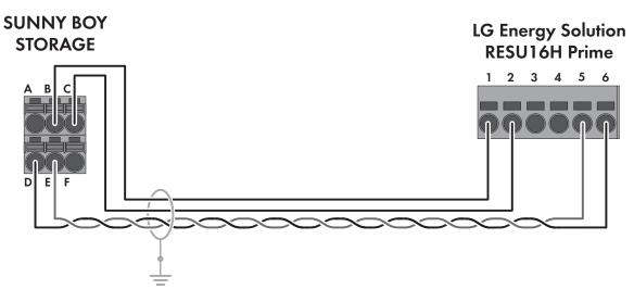
Figure 12: Cabling plan SBS3.8-US-10 / SBS5.0-US-10 / SBS6.0-US-10 with RESU16H Prime
