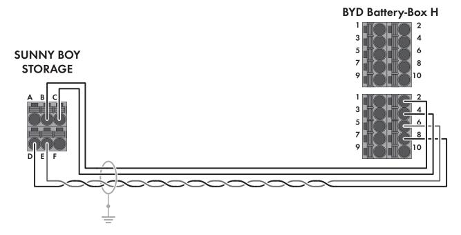
Figure 7: Cabling plan SBS3.7-10 / SBS5.0-10 / SBS6.0-10 with Battery-Box H  $\,$
