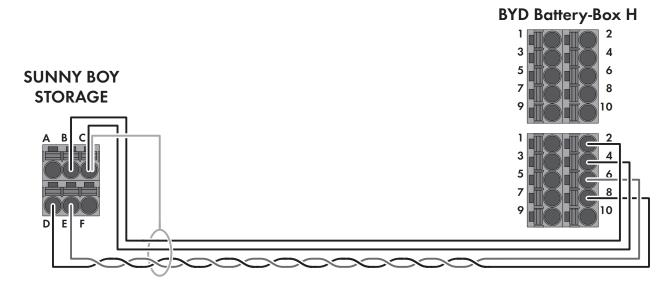
Figure 2: Cabling plan SBS2.5-1VL-10 with Battery-Box H
