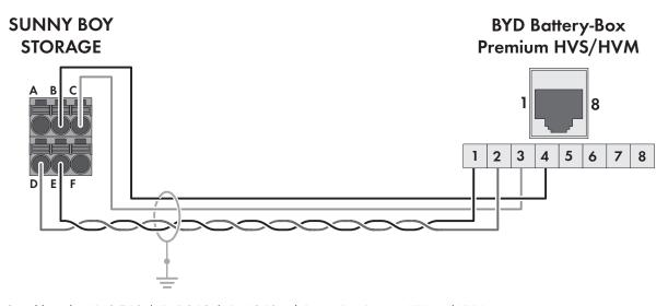
Figure 8: Cabling plan SBS3.7-10 / SBS5.0-10 / SBS6.0-10 with Battery-Box Premium HVS and HVM
