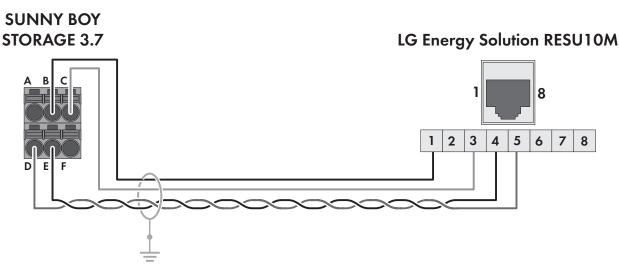
Figure 5: Cabling plan SBS3.7-10 with RESU10M
