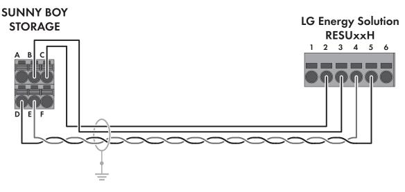
Figure 10: Cablin plan SBS3.8-US-10 / SBS5.0-US-10 / SBS6.0-US-10 with RESU7H / RESU10H
